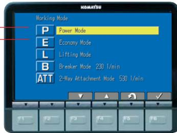
**E mode** – Economy or fuel priority mode further reduces fuel consumption, but maintains the P-mode-like working equipment speed for light duty work.
