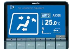
instruments on the large LCD. The bi-level control function keeps the operator's head and feet cool and warm respectively. This improved air flow function keeps the inside of the cab comfortable throughout the year. Defroster function keeps front glass clear.
